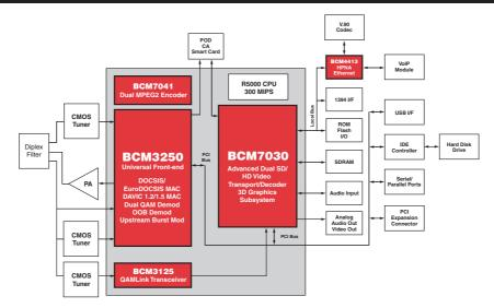
The Broadcom **BCM93740** is an advanced set-top box development platform supporting high definition television (HDTV), dual standard definition decoding and broadband cable modem internet access. It is a highly integrated, cost-effective design built on the latest generation of Broadcom silicon and software offering low risk and quick time-to-market for the next generation of interactive set-top boxes.
